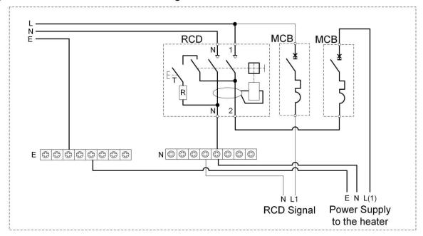
3 Phase Connection of RCD signal to dedicated Power Board for Evolution2 Heater
