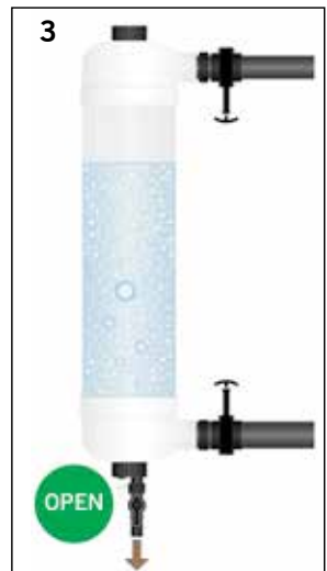
3. Open waste valve tap
