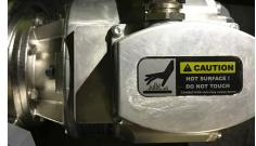
Be careful: the surface of the pump can be very hot (up to 75 °C). Do not touch it directly before checking the surface temperature. For the pump itself, this temperature is normal and no problem. Always ensure good ventilation around the pump.
