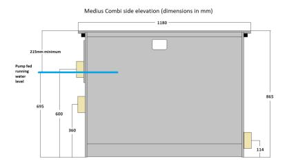
Also in pump fed installations, the filter needs to have the water level set at this height by an external standpipe return. The following diagram shows this layout —
