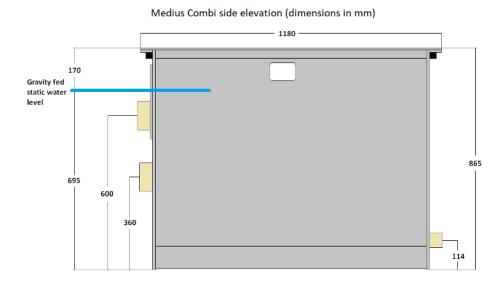
The diagram shown equates to static water level (no pumps running) almost brimming the waste tray in the drum. This gives maximum coverage of the drum screen. There should be as little restriction as possible in the 4" pipework before the filter.
