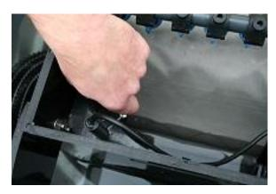
**For gravity fed units** the sensor is on the clean side of the drum. This sensor is triggered when the micron screen becomes dirty and blocked and the water level starts to drop as not enough water is able to get through.
