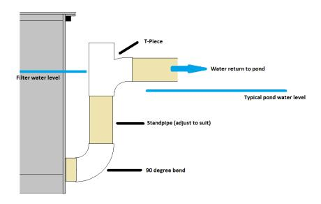
In short runs, the return pipe should be no less than 3" in diameter. For longer runs, 4" is preferable. In the magna, 2 x 4" runs would be advisable. In the above diagram, a vertical standpipe governs the height of the water in the filter. A t-piece then returns the water to the pond. A t-piece is recommended as it stops syphoning and/or surging in the return pipe on longer runs.
